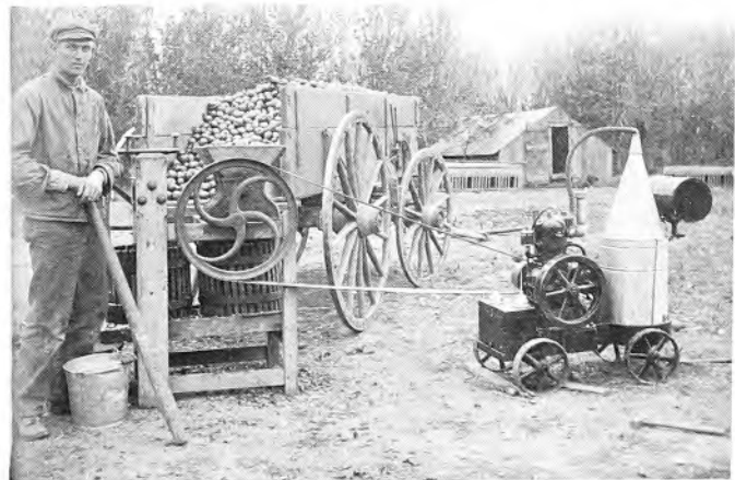
Cider press, powered by a portable 4-HP gasoline engine (about 1915).
